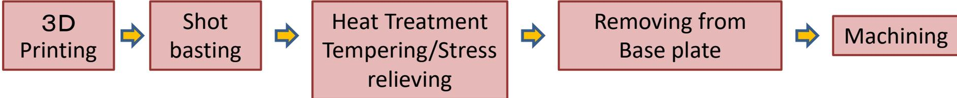
Typical mold manufacturing process using DAP™-AM HTC.
