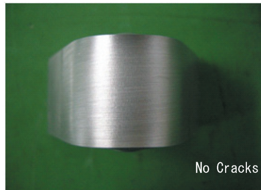
Fig. 13. Results of copper-copper sulfate-16 % sulfuric acid test of DNM140-HCR
