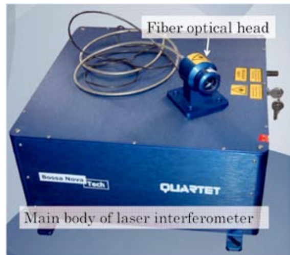
Fig. 22. New line of laser interferometer with fiber optical head.
