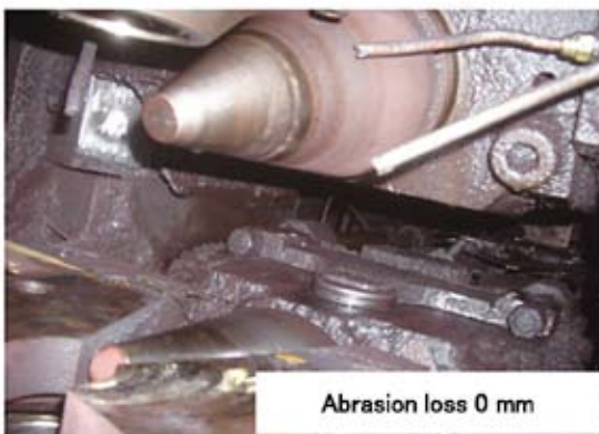
b) KV overlaid axial roll after two weeks
