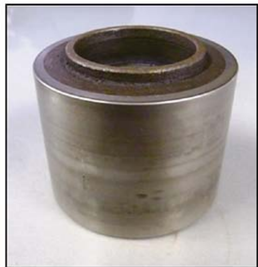
b) KV overlaid measuring roll after 6 months
