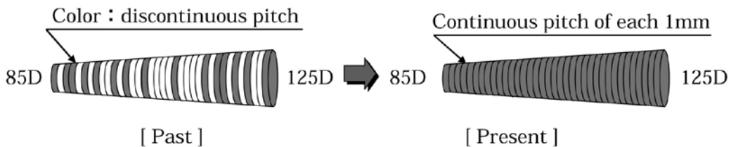
Fig.1. Change in the Rolling Size pitch.
